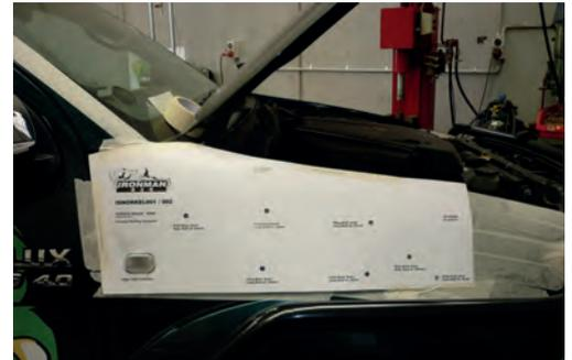
5. Using a felt tipped pen, mark all holes through template onto mudguard. Remove template.
