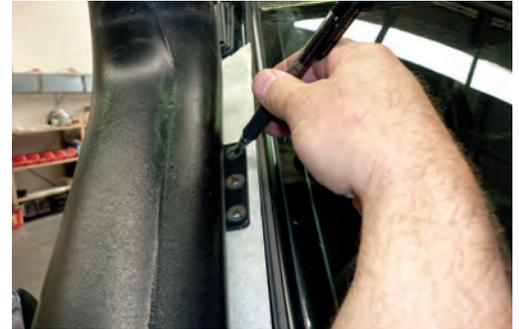
10. Drill mounting holes in pillar to 7.5mm. Apply silicone sealant. Insert mounting plugs and attach mounting bracket using three self tapping screws provided (When drilling mounting holes, only drill through outer skin and no further.)
