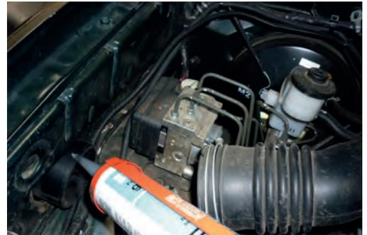
15. Refit cyclonic air intake and air intake hose to air cleaner.
