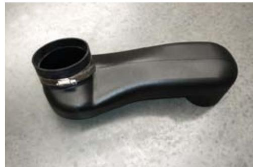
13. Place air entry duct under mudguard and align rubber joiner with snorkel hole.
