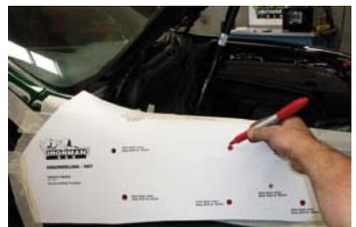
6. Using a hole saw cut a 95mm hole for snorkel duct and drill all mounting holes to 16mm.
