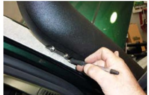
10. Hold snorkel bracket in position and mark four mounting holes on pillar. Drill mounting holes to 7.5mm.
