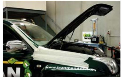
4. Tape template to mudguard making sure it is lined up with top of mudguard (bonnet opening) and rear of mudguard (door opening).
