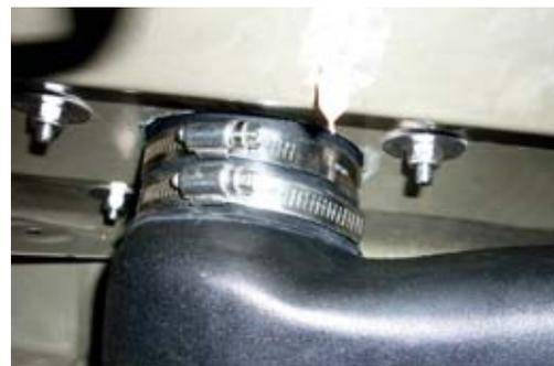
15. Secure to vehicle using M8 Nylock Nuts and Body washers. Attach to pillar mounting bracket using M6 Bolts. Secure rubber joiner to snorkel with hose clamp.
