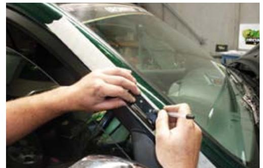
11. Apply silicone sealant to holes. Insert mounting plugs and attach mounting bracket to pillar using self tapping screws provided.
