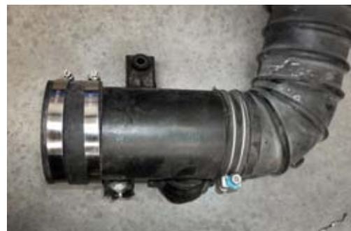
17. Refit factory air intake duct to engine bay. Attach rubber joiner to air entry duct and tighten all hose clamps.
