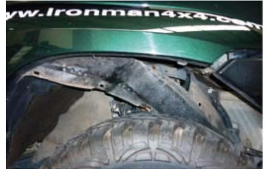
3. Apply masking tape to right hand front mudguard and windscreen pillar.
